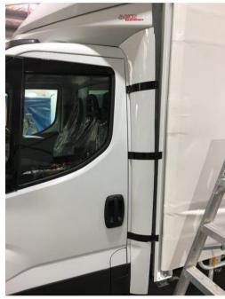
4. Repeat the process for the extenders. Hold the extenders in position using tape.
