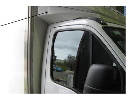
1. Place the roof device on cab roof and hold the cab extenders in position. This will give you the working area of the cab to be prepared.
