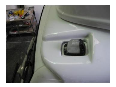
5. The rear of the clearance lights should sit approximately 10mm from the rear edge of the clearance light recess (Refer photo). Once the Fuelscoop PLUS is in position, peel the protection film off all the double sided tape and then remove the packers. Press down firmly to ensure the tape adheres to the cab roof.
