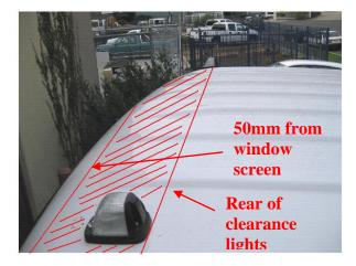
2. Clean the cab roof using Tite-R-Bond (supplied) in the areas as per photos above. Use a lint-free rag and ensure the bonding area is completely free from dust.
