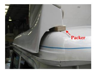
4. Lift the Fuelscoop PLUS onto the cab roof and place packers under the front and rear corners. This will allow you to move the Fuelscoop PLUS into position without the double-sided tape touching the cab roof.
