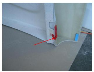
3. Peel the protective film from the double sided tape at each end and tape this film to the outer surface of the Fuelscoop PLUS. This will make it easier to remove the protective film once the Fuelscoop Plus is sitting in position.
