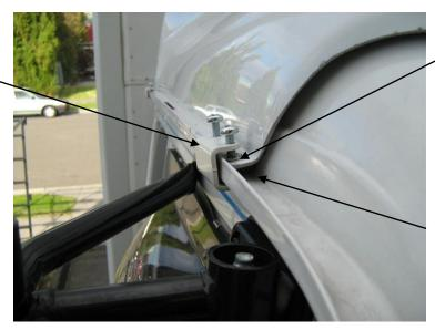
Clamp Plate (between Clamp Bracket and scoop)
