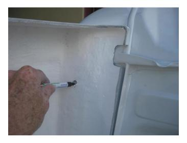
2. Mark the nutsert hole on the rear of the cab.
