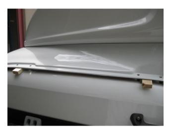
5. Place Fuelscoop Plus on cab roof in position. Sit Fuelscoop Plus on packers so the double sided tape does not touch the roof.
