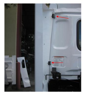
4. `Replace the extender and bolt it to the cab using the 8mm set screws into the nutserts.
