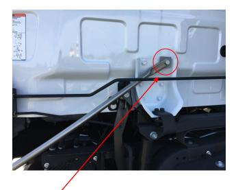
10. For the LHS lower extender brace, remove 10mm bolt and fasten lower extender braces to the cab and extender with the bolts, washers and spacers provided.
