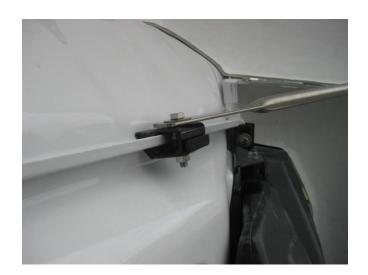
12. The extender upper braces are clamped to the rear gutter.
