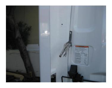
Hold the near side extender in position and clamp it to the vertical rib on the rear of the cab.
