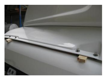
6. Loosely screw 8 x 40mm bolts in position. You may need to enlarge some holes so the bolts fit.
