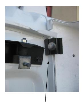
6. Ensure the upper clamp set is as close to the gutter as possible.
