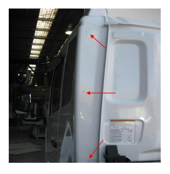
3. Remove the extender. Drill and fasten the 3 nutserts down the rear of the cab.
