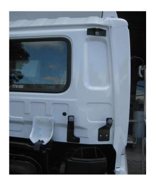
5. Remove the air intake and repeat the procedure for the RHS lower extender.
