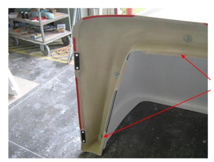
Peel protection film off completely on the inside of the scoop.
