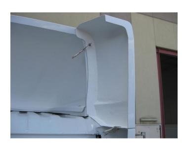
13. Clamp the upper extenders in position, then drill and bolt them to the rear of the roof device and top of the lower extenders.
