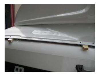
5. Place Fuelscoop Plus on cab roof in position. Sit Fuelscoop Plus on packers so the double sided tape does not touch the roof.
