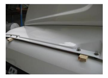
6. Loosely screw 8 x 40mm bolts in position. You may need to enlarge some holes so the bolts fit.
