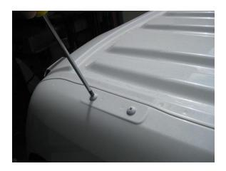
1. Remove 8 bolts in cab roof.
