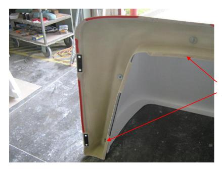
Peel protection film off completely on the inside of the scoop.
