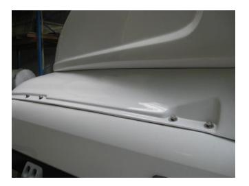
7. Remove protective film from the double sided tape and allow the Fuelscoop Plus to fall to the roof.
