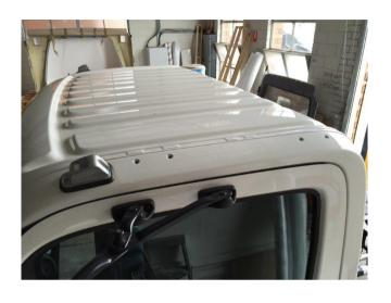
1. Remove the 8 bolts from cab roof.
