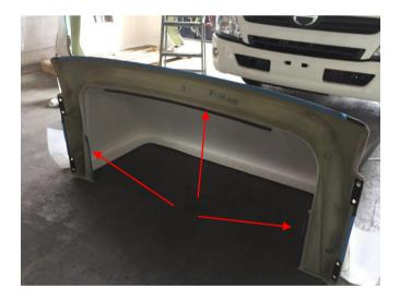
5. Peel protection film off the double sided tape on the 3 inner strips.
