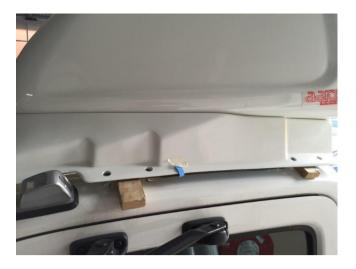
7. Place some spacer blocks on the cab roof between each tapped hole. Place the Fuelscoop in position on the cab roof ensuring the kit does not contact the roof.
