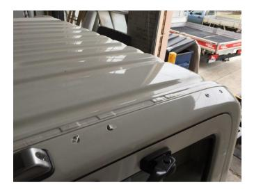
4. Place sealant in and around the 8 tapped holes in the cab roof.
