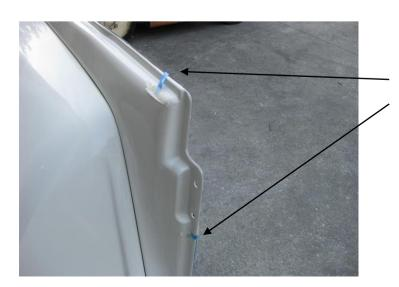
6. Slightly peel the edges of remaining double sided tape strips so they stick outside the part.
