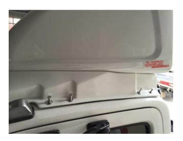
9. When all bolts are in loosely, peel the protection film from the tape and remove the spacers. Gently lower the Fuelscoop onto the cab roof.
