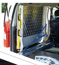
**EASY** is ideally suited to smaller vans, or applications where a ramp is important, but not required continually. Easy is mounted at right angles to the rear, and/or side door. When released it slides out, rotates right to lock position and is then unfolded. Easy is 80cm wide and available in lengths of 2m, 2.5m and 3m. It is rated at 300Kgs.
