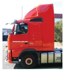
1. FUELSCOOP roof deflectors and Full Aero-Kits are brand and model specific, matching perfectly with the cab design. The roof mount system picks up on factory installed mount point, ensuring a no-risk installation. For full kits lower cab extenders are interference fit and the upper extenders join roof device to cab extenders.
