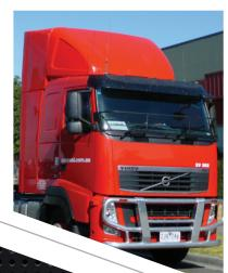
3. A frontal view of Fuelscoop exposes a 'cut' that redirects the airflow outwards causing a 'streaming' affect. With the Full Aero-Kit this intensified airflow stream passes over the extenders to a final 'kick' at their rear edge, assisting the flow onto the trailer, improving the truck's safety, increasing performance and improving fuel economy.
