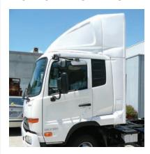
1. Fuelscoop Full Aero Kits are brand and model specific, matching perfectly with the cab design. The roof device has a moulded base mounting system that picks up on UD factory installed mount points, ensuring a no-risk installation. The lower cab extenders are interference fit and the upper extenders join roof device to cab extenders.
