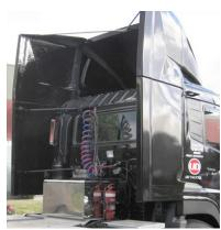
2. Fuelscoop Full Aero-Kits, in addition to their overall visual and performance appeal, are without excessive weight. The total weight of under sixty kilograms is achieved by means of design. This proven design means that the need for heavy steel brackets is eliminated. The load is spread over the total mounting surface and is trouble free.
