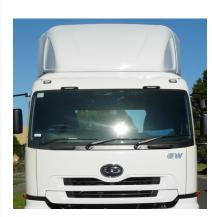
3. A frontal view of Fuelscoop exposes a 'cut' that redirects the airflow outwards causing a 'streaming' effect. With the Full Aero-Kit this intensified airflow stream passes over the extenders to a final 'kick' at their rear edge, assisting the flow onto the truck body, improving the truck's safety, increasing performance and reducing fuel consumption.
